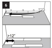
Start the second row with the leftover cut part of the last plank of the previous row. This small plank should measure at least 12".
