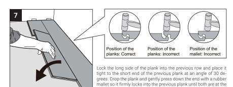
NOTE: If you notice both planks aren't at the same height or are not well locked together, please follow the disassembling instructions at the end of installation steps; disassemble and check if any debris stuck inside the lock is obstructing
