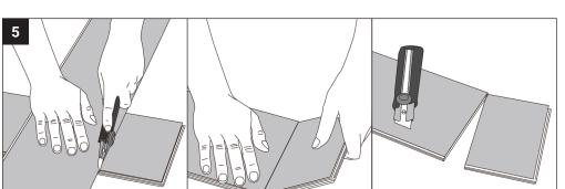
To cut the plank, use a simple utility knife and ruler, and with the top side facing up, cut heavily and several times on the same axis. The knife will not go through the surface but make a deep cut. You can then lift one half of the plank using your other hand to hold down the second placing it very close to the cut. The plank will split naturally.
