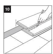
To lay the last row: position a loose board exactly on the top of the last row laid. Place another board on top, with the tongue side touching the wall. Draw a line along the edge of this board, to mark the first board. Cut along the edge of this board to mark the first board. Cut along this line to obtain the required width. Insert this cut board against the wall. The last row must be at least 2" wide
