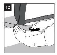
Door molding and skirting: lay a board (with the decorative side down) next to the door molding and as shown in the figure. Then slide the floorboard under the mold-
