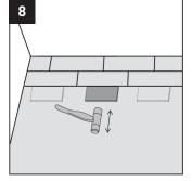
After finishing the installation of the row, use scrap pieces and a small hammer or rubber mallet to gently tap the planks into the click of the previous row to make sure they are tightly clicked together and make sure there is no gap between the long side of the planks installed. ANY GAPPING CAN COMPROMISE THE WHOLE INSTALLATION.
