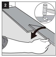
Second plank, first row. Drop the plank and gently press down the end with a rubber mallet so it firmly locks into the previous plank until both planks are at the same height. Make sure both planks are perfectly aligned.
