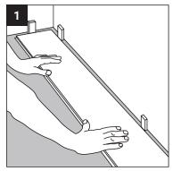
After thoroughly cleaning the subfloor, you should begin laying in the left-hand corner. Place the floorboard ¼" from the left wall. Use spacers between the wall and the floorboard
