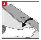
Starting from the corner closest to the previous plank, fold down towards the center in a single action.
