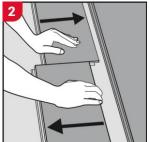
Disassemble each plank by sliding the short ends horizontally. Never fold up the plank as this will damage its locking profile.
