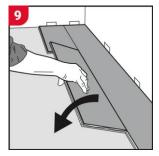
Second row, second plank Gently place the plank close to the short end of the previous plank and fold down in a single action.
