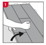
Separate the entire row by carefully lifting up and releasing it. Fold up the row and release the whole long side.
