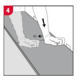
Press down firmly and listen for the click that means it's locked in place. No tapping is required.
